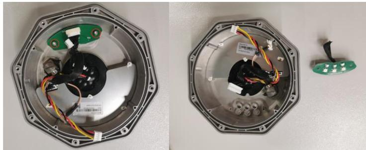
10. Remove RF connector, use wrench to unscrew the hexagon nut
