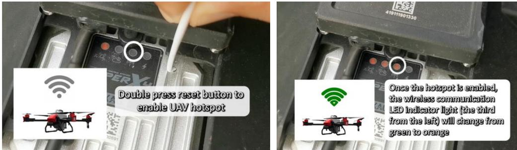
**Scenario:** double press reset button; the wireless communication light does not change to orange.
