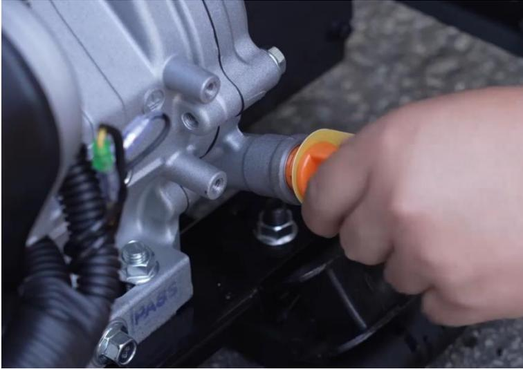
The 1<sup>st</sup> service should be taken placed after 20 accumulated operation hours.
