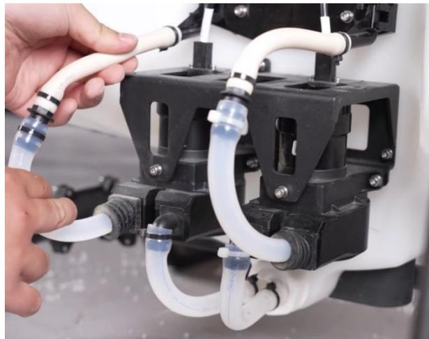
7. **Check Hose Manually and visually inspect hose to check whether it is broken or worn.**
