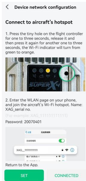
6. Double press the reset button on flight control
