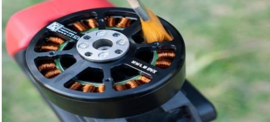
A close-up photograph of a motor's stator. A yellow brush is being used to clean the copper windings. The motor is black and red. The background is a blurred green area.                                                                                    |
