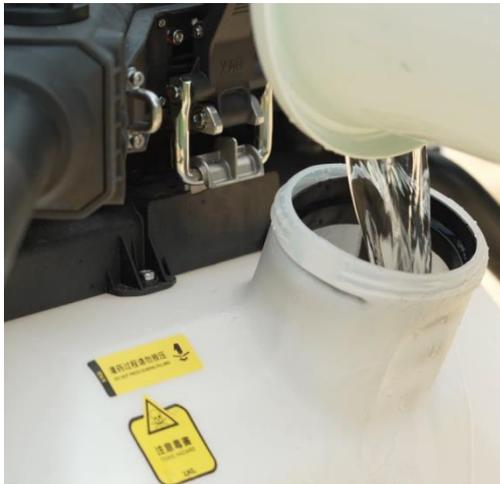
Make sure the remaining volume has enough liquid to perform manual spray test. You are allowed to set the individual pump flow rate and nozzle speed. The speed and current measurement of S1 and S2 should be very close.
