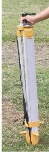
2. Adjust the screws to extend the legs of tripod
