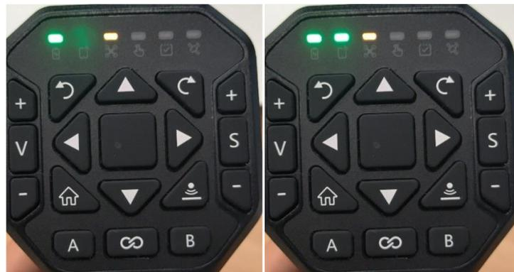
3rd led Flashing yellow: pairing mode or connecting to local wifi
