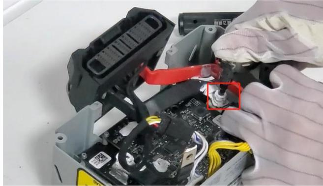
Step 3: Remove the battery plug
