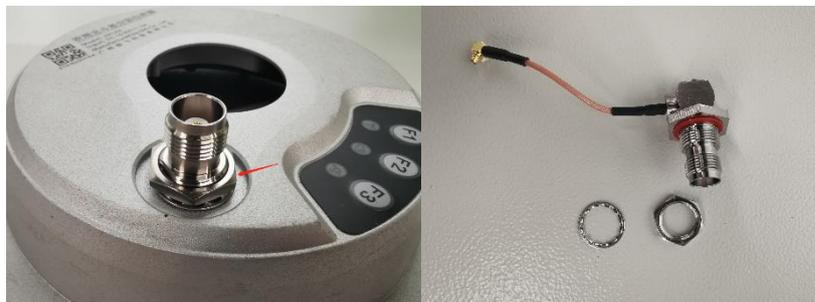
11. Remove GNSS fixture column and its gasket
