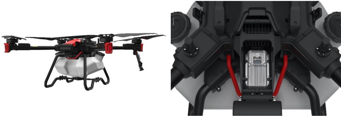
SuperX4 Pro Flight Control is used in P100.
