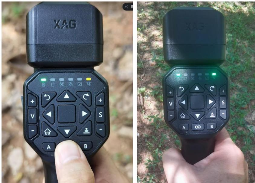
2. Make sure that smartphone is connected to ACS2 hotspot, but it does not matter if the ACS2 has internet access or not. (The second led can be on or off)
