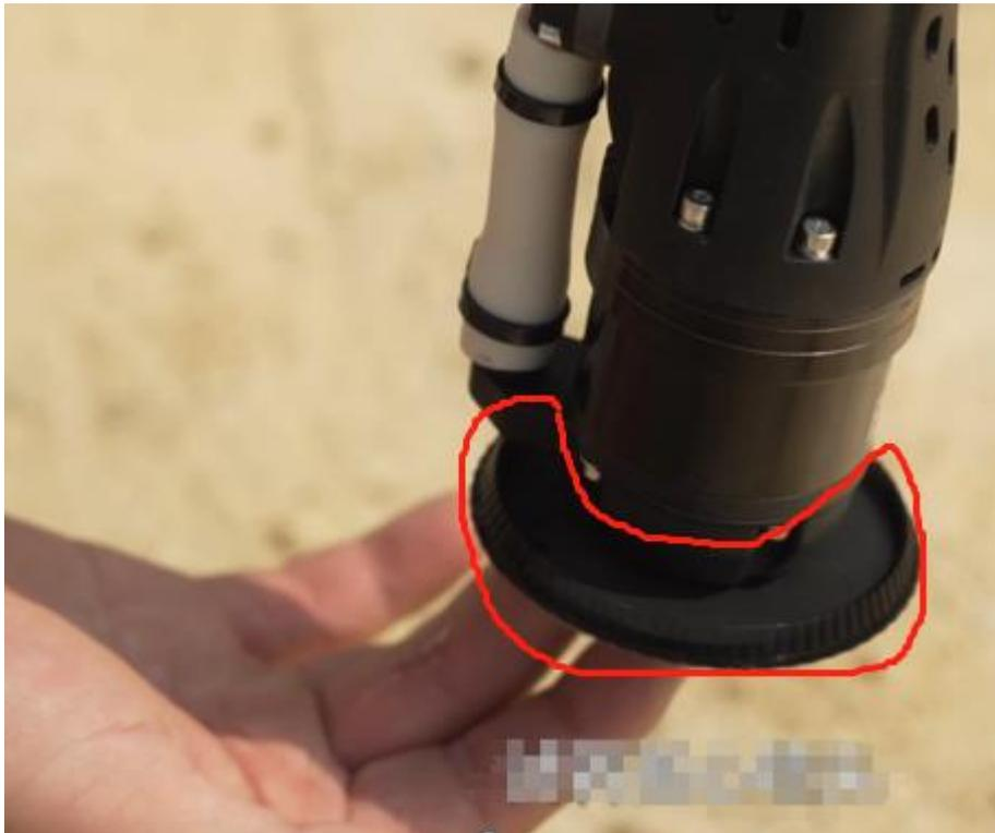
Check the RTK antenna installation
