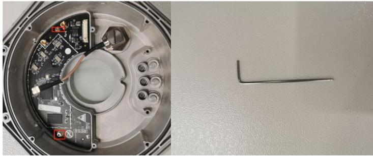
Note: The thermal conductive silicone pad pastes between the WIFI board and the bottom shield. It makes the WIFI board difficult to be removed from the bottom shell. In this case, we can use a heater to warm up the bottom shell for 1~15 minutes. Then plug on the cable, grab the cable, and slowly pull the WIFI board away from the bottom shell
