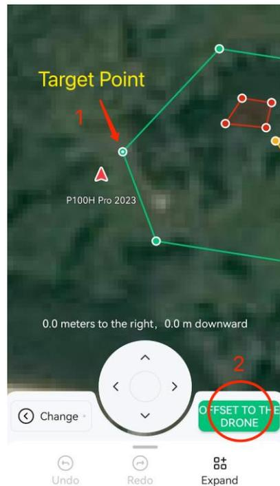
5. Then the field boundary will move according to target point, which will match to the drone position (drone symbol), Tap confirm button on the screen to complete offset correction. Now the relative position of the drone and the field is correct.
