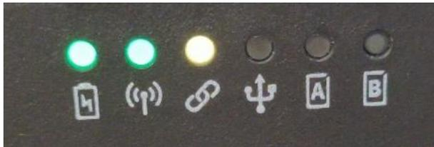
Make sure the first 3 leds of the ARC3 Pro are all on
