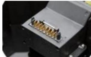
10. Inspect Radar: Visually check whether the main front radar mount is deformed. If there is deformation, it should be replaced immediately. The deformation of the radar mount will affect the radar detection ability. Radar Cable should be on the left, reinstall radar if incorrect.
