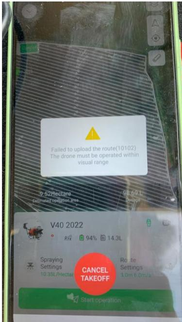
Analysis: The location is disabled. The app does not know the user's location. Thus, it fails the safety check because it can't calculate the distance between drone and user's smartphone.
