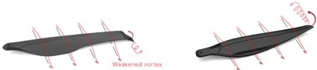
XAG propellers tips. Some tip up while others tip down. But both are proven to weaken vortex.
