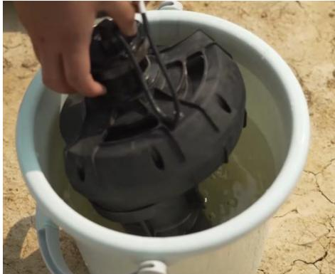
Use clean water to rinse spiral feeder. It's recommended to use high pressure water gun.
