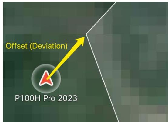
3. The offset correction tool will then show up with all the points of the field displayed. You can either use the arrows to fine tune the position of the field map (each click moves 0.5 meters), or just select the target point of the map.
