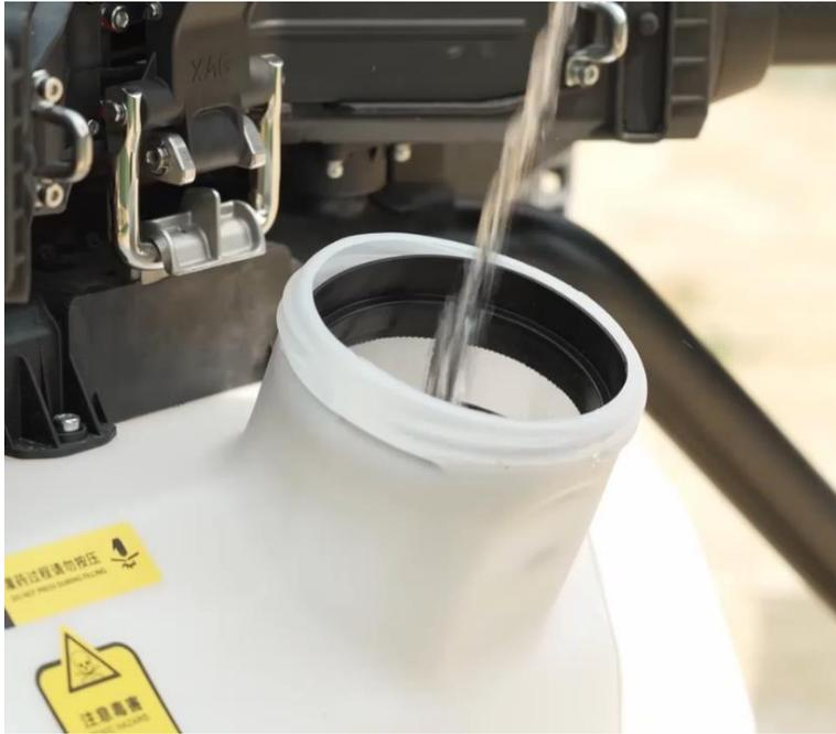
Emit the water from liquid tank to clean spray system again.
