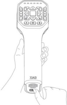
Optional: To eliminate the influence of 4G and make sure that ACS2 WIFI hotspot is enabled, we can **REMOVE** the SIM card
