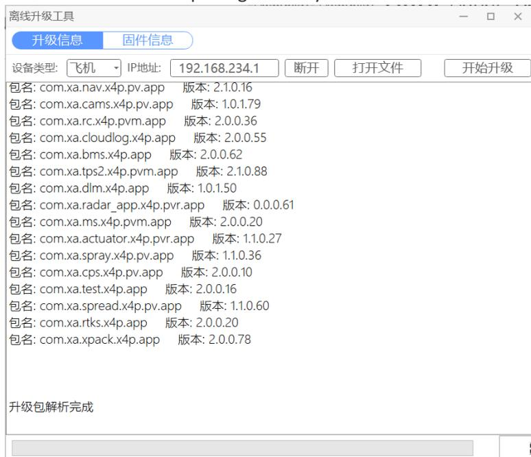
8. After clicking the “开始升级 ” (“Start Update”) button, the device will begin to update all firmwares in the package, and the progress bar will display the progress of uploading and updating.
