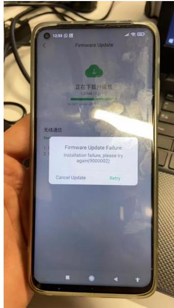
**Analysis:** This error could be caused by significant network latency. The XAG server is based in China, thus the user who are far from China, will evitable suffered from this.
