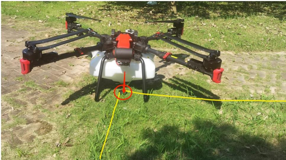
2. Go to the operation page and select the field you are going to work on, you will find the UAV symbol is not exactly at the corner. There is a deviation from the point where it should be and you are required to perform offset correction. Tap “Offset correction” button on the screen
