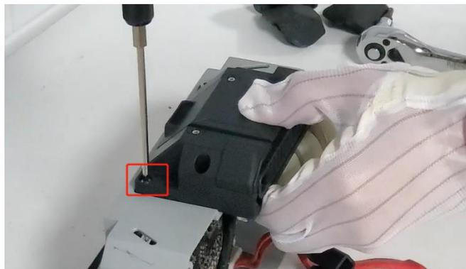
Step 2: Remove one screw on the positive and negative copper terminal.
