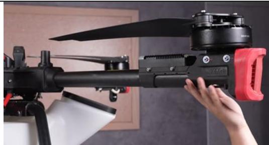
9. **Inspect the joint of motors and base from loosening**
