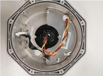
12. Remove EMI shield, unscrew 5 screws
