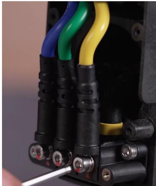
5. **Inspect the ESC screws from loosening**
