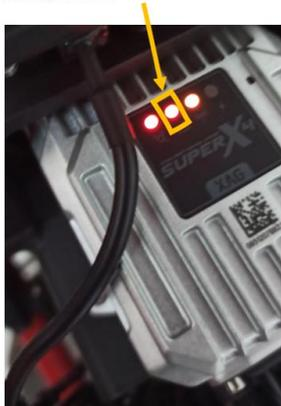
Flight control is connecting to internet through 4G as the 2<sup>nd</sup> light indicator (remote server) is in green.
