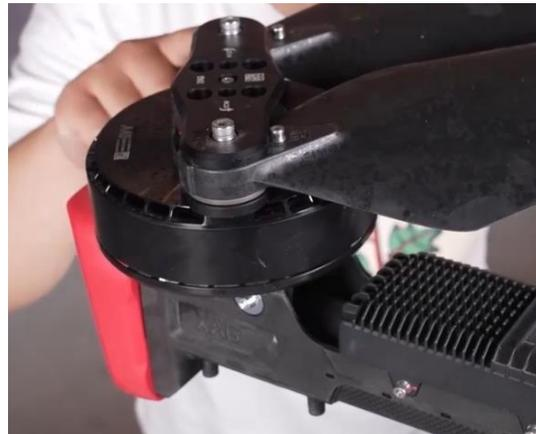
12. **Inspect its bearings from loosening or abnormal sound. Rotate the motor to check the motor bearings**
