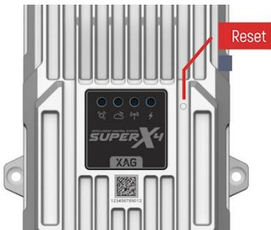
WIFI and Cloud indicator turns into orange, shut down the UAV, wait for more than 5 minutes, start the UAV again. The UAV is supposed to quit LNT networking mode.
