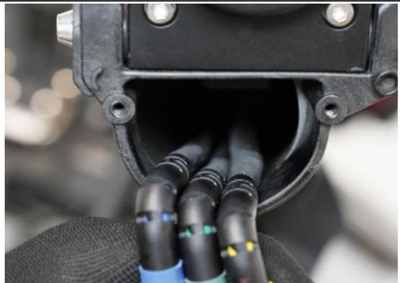
4. Inspect the cable connection of motors and ESCs from loosening.
