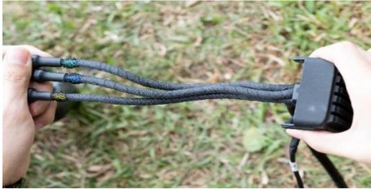
A close-up photograph showing a person's hands holding three black three-phase wires connected to an ESC. The wires are being inspected for wear or damage. The background is a grassy area.                                                                 |
