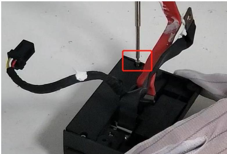
Step 2: Remove the battery plug case
