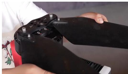
11. **Inspect the screws (motor/clip) from missing or loosening**
