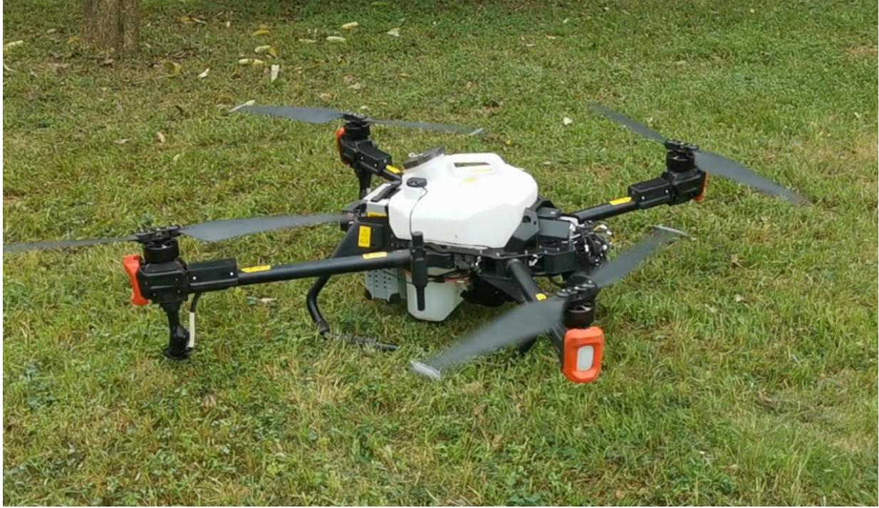
For good practices, idle test should be performed regularly. If the UAV is recently repaired or under maintenance, it's necessary to perform idle test before flight mission.
