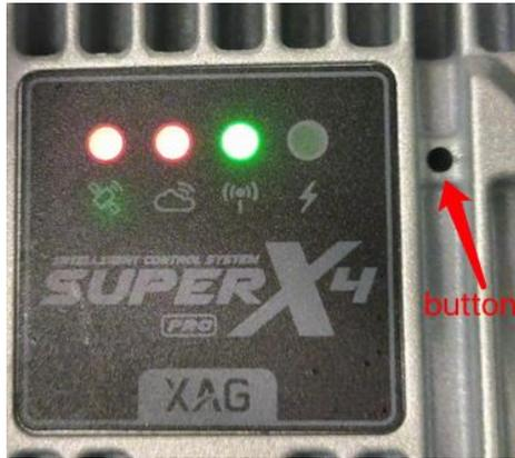
1. For P100H, release reset button of flight control when WiFi light indicator (the third light of flight control) alternates between green and red; Arm light slowly flashes yellow.
