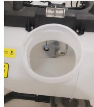
9. Check Charging System Connector: Inspect the charger and water tank plug (if using cooling tank) and ensure the plugs are clean and free of debris. Clean any debris and ensure all electrical plugs are dry before use.
