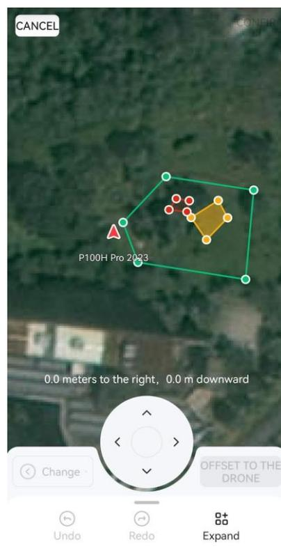
4. Select the target point (field boundary reference point), and then tap “Offset to the drone” button
