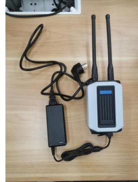
**Turn on LNT:** Long press power button for 2 seconds, release the power button when the 1<sup>st</sup> light indicator (Power) illuminates in green. Wait for 1 minute. The LNT is under initialization when 2<sup>nd</sup> / 3<sup>rd</sup> / 4<sup>th</sup> light indicators (WAN/WLAN/System) are flashing. Once all the light stop flashing and illuminate in green, the LNT is ready to use.
