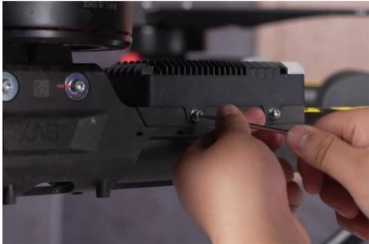
A close-up photograph showing a person's hands using a screwdriver to inspect a screw on the black fuselage of a drone. The screw is being turned, and the person is looking closely at it. The background is blurred.                                        |
