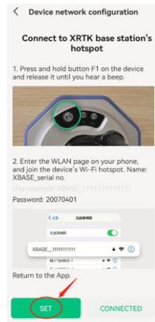
8. Under smartphone WLAN setting, Connect XRTK4 hotspot. The XRTK4 hotspot SSID is XBASE\_[serial number], and the password is 20070401. It will take approximately 20 seconds until the XRTK4 hotspot appears.
