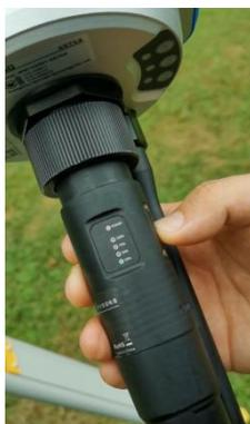
7. Insert XRTK4 into the tripod fixture slot, lock the clamp
