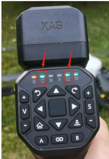
4. Make sure that smartphone is connected to LNT hotspot, but NOT the 4G network
