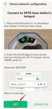
6. Under smartphone WLAN setting, Connect XRTK4 hotspot. The XRTK4 hotspot SSID is XBASE\_[serial number], and the password is 20070401. It will take approximately 20 seconds until the XRTK4 hotspot appears.
