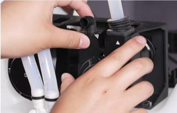
Inspect the lubrication between peristaltic pump internal rubber tube and plate synchronizer
