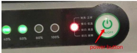
1. For P100H, release the battery power button when the arm light slowly flashes yellow, and the WiFi light indicator (the third light of flight control) alternates between green and red..
